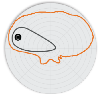
Figure 5. T750 5GHz Elevation Antenna Patterns
