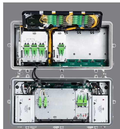
EDFA Optical Amplifier Modules in Chassis (open view)
