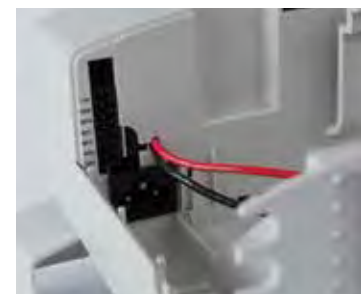
Output Cable Connection
