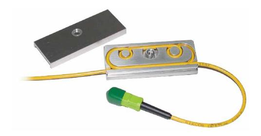
\* The Olson Technology, Inc. **Model OTOA-1000** provides 1dB though 7dB of step-variable attenuation (i.e. @ 1dB steps) for 1310nm signals via standard simplex 9/125 yellow nonplenum riser jacketed singlemode fiber cable. Results may vary with other wavelengths and types of fiber cable.
