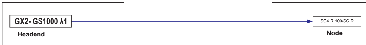
Figure 1: Transmitter with No EDFA to Node
