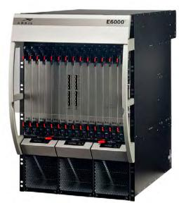
The E6000 CER provides cable operators with unprecedented efficiencies in DC power consumption per downstream channel. This leads to reduced powering and cooling requirements for the operators' facilities, which can provide significant savings in operational and capital expenditures.
