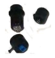
The **ATT100** series are ideal for simulating cable loss for lab testing of link power margin or reducing power in links where receivers are being overloaded. The ATT100 variable attenuators are of the gap-loss type. Pulling the connector end faces apart induces the loss. If you are using these attenuators in a laser or CATV system, you should use the ATT120 with a FC/APC connector, which have very low return loss even when unmated.
