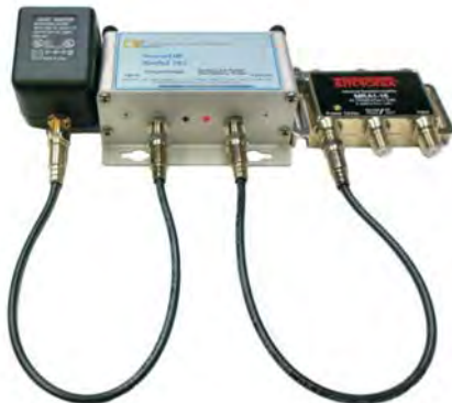
Figure 4 - NeverOff Model 101 Powering an Antronix MRA1 with Antronix wall supply.
