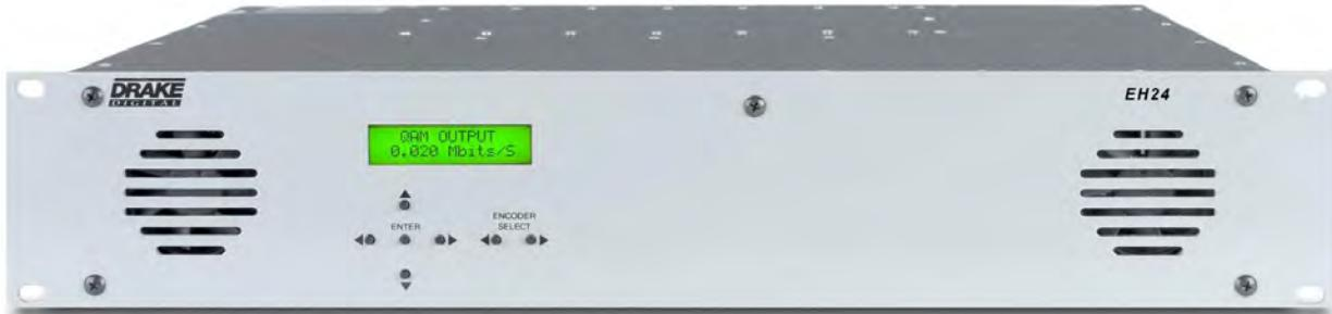
The Drake Digital™ EH24 platform is a 19" rack-mountable 2RU chassis that accepts up to six real-time Drake Digital™ SDE24 MPEG2/MPEG4 video encoder modules. The Drake Digital™ SDE24 MPEG encoders contain two video encoders each, enabling the Drake Digital™ EH24 to accept 12 different video input sources/channels to be multiplexed after encoding (when populated with six SDE24 modules). The EH24 accepts any number of SDE24 modules (1-6) adding two video programs per module..
