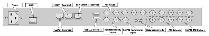
**Power:** 70 – 240 VAC switching power supply; standard 3-pin computer power plug.
