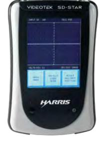
The new Videotek® SD-STAR™ is a handheld, battery-powered monitor and test generator for SD-SDI and analog composite video signals. The unit provides multiformat functionality and versatility, setting it apart from other handheld test products on the market.
